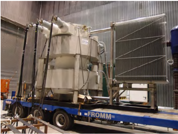
Figure 11 FCL during Thermal Test at IPH, Berlin
